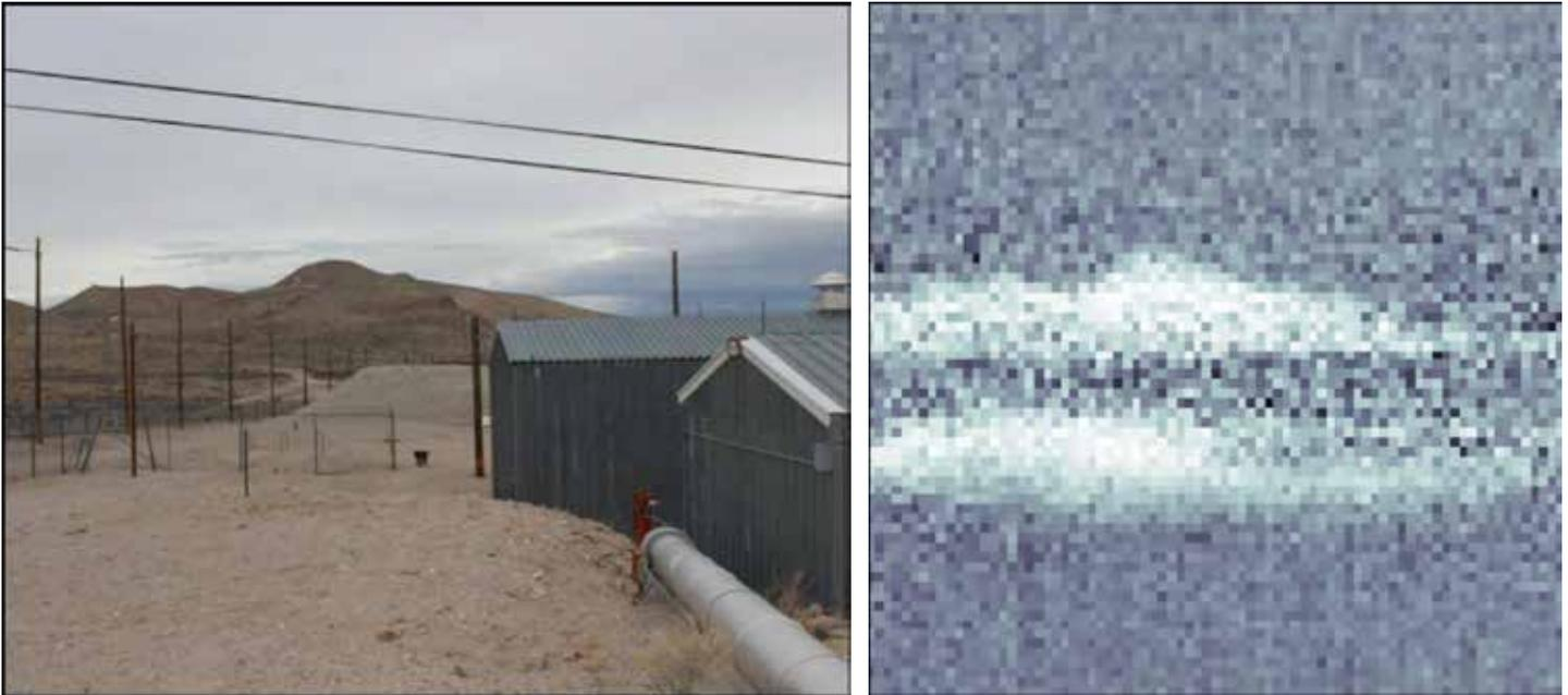
**Figure 6:** Photo (left) of mountain being imaged (right) from horizontally traveling muons in telescopic mode. The lighter area in the top portion of the figure on the right represent the mountain in the photo on the left. The lighter area in the bottom portion of the figure on the right is due to “noise” from muons detected from the opposite direction.
