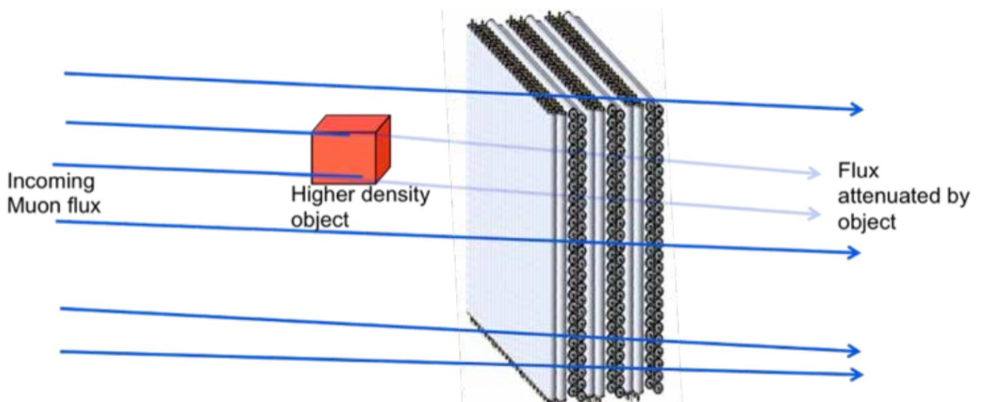
**Figure 3:** Telescopic imaging mode.
