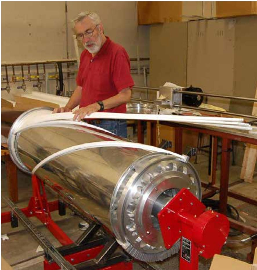
**Figure 1:** The late John McGill wrapping the first helical layer of scintillator strips for tracking muons on the hollow inner core of the detector.
