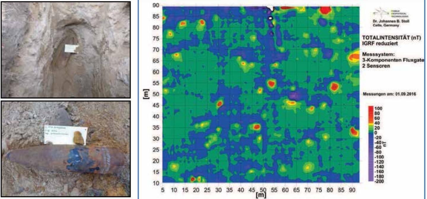
**Figure 6:** On left side are photographs of a 155 mm “grenade” removed from site as a result of the magnetic map (on right) created using the MGT dual sensor vector magnetometer and a UAS.
