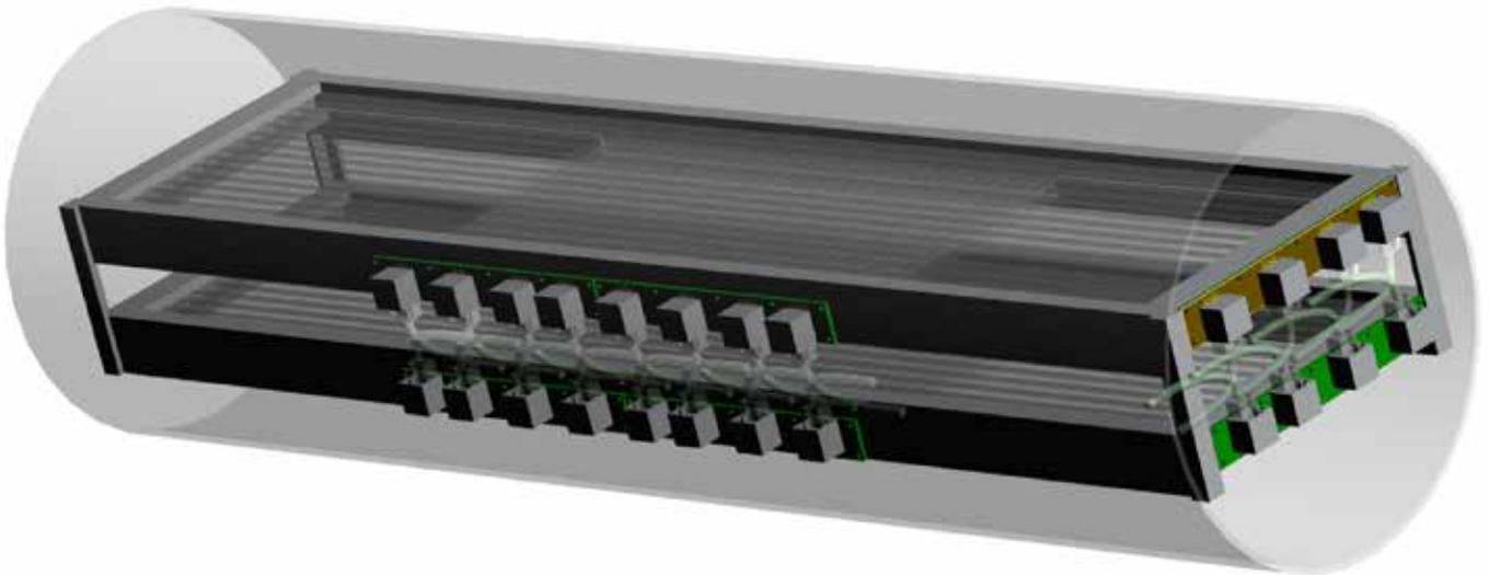
**Figure 5:** The PNNL Borehole Muon detector consists of 30 horizontal long scintillating rods in two layers and 60 short perpendicular rods in two layers, optical fibers, light sensors, and electronics to detect each muon that passes through the device. Several computer simulations of muons trajectories have been performed to select the optimal geometry of the different layers. The detector counts the muons but also determine their trajectories which is required to build a 3D density image.
