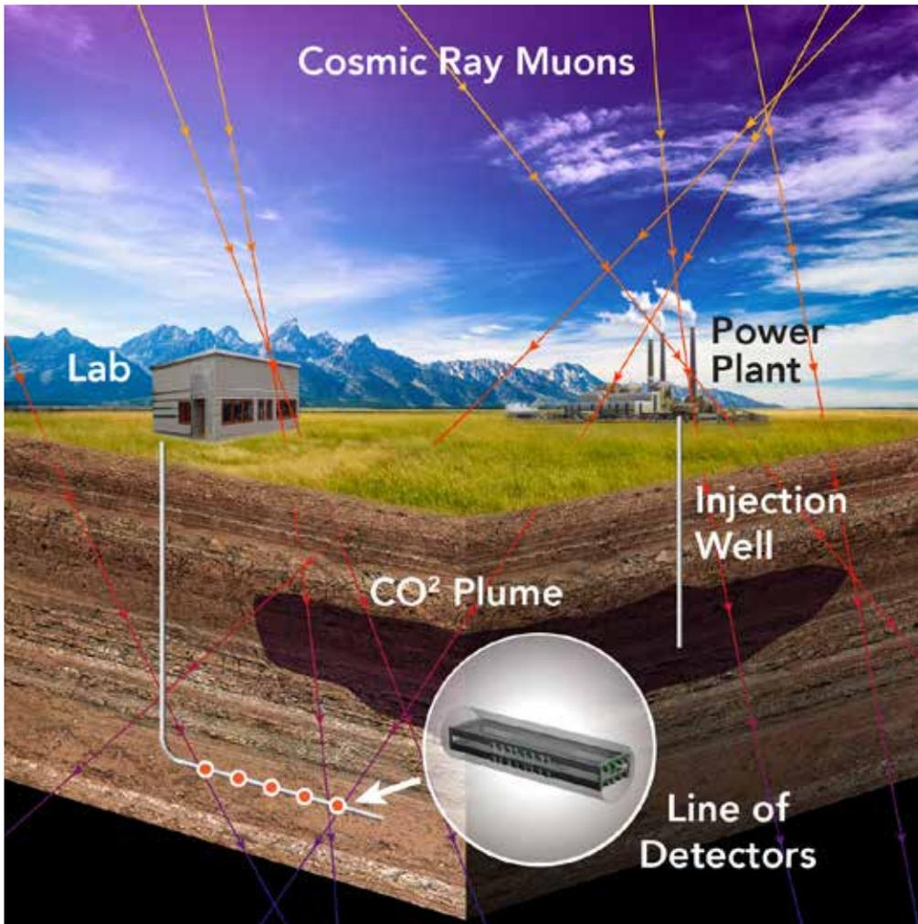
**Figure 4:** Conceptual representation of monitoring of a CO<sub>2</sub> geological storage by muon tomography. A series of PNNL borehole detectors are deployed permanently beneath the reservoir to monitor the change in density due to the replacement of brine by CO<sub>2</sub> in the geological formation.
