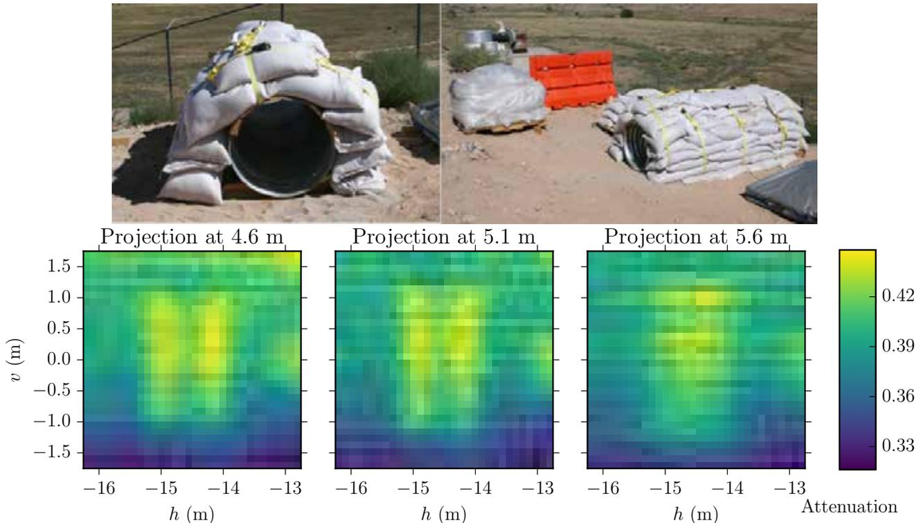
**Figure 5:** Closeup of arch projection and images of actual arch created with sandbags. The hollow center is clearly visible, joining together in higher projections.
