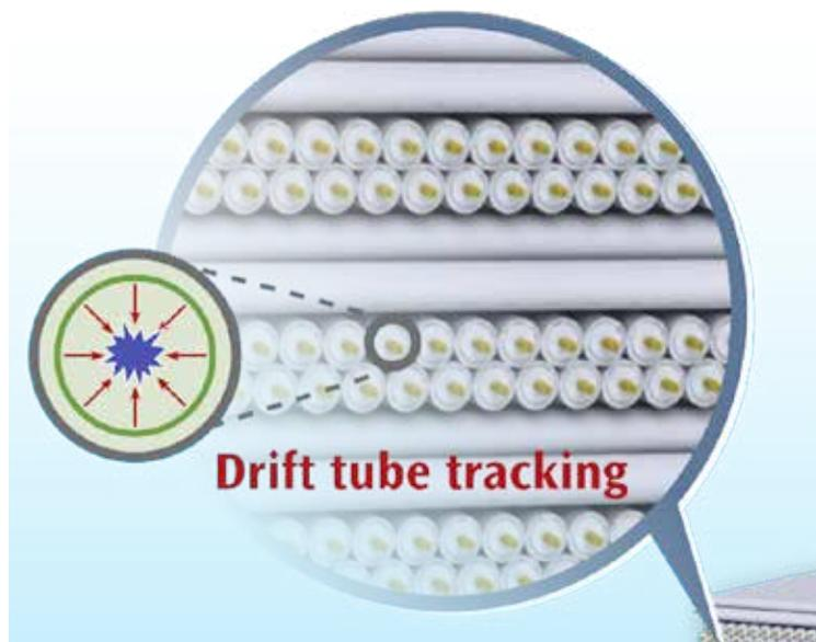
**Figure 1:** Drift tube detector: series of drift tubes in X and Y orientations. The expanded tube show electrons drifting toward the wire after the gas in the tube is ionized by a passing muon. The muon would have hit this tube tangent to the green circle.
