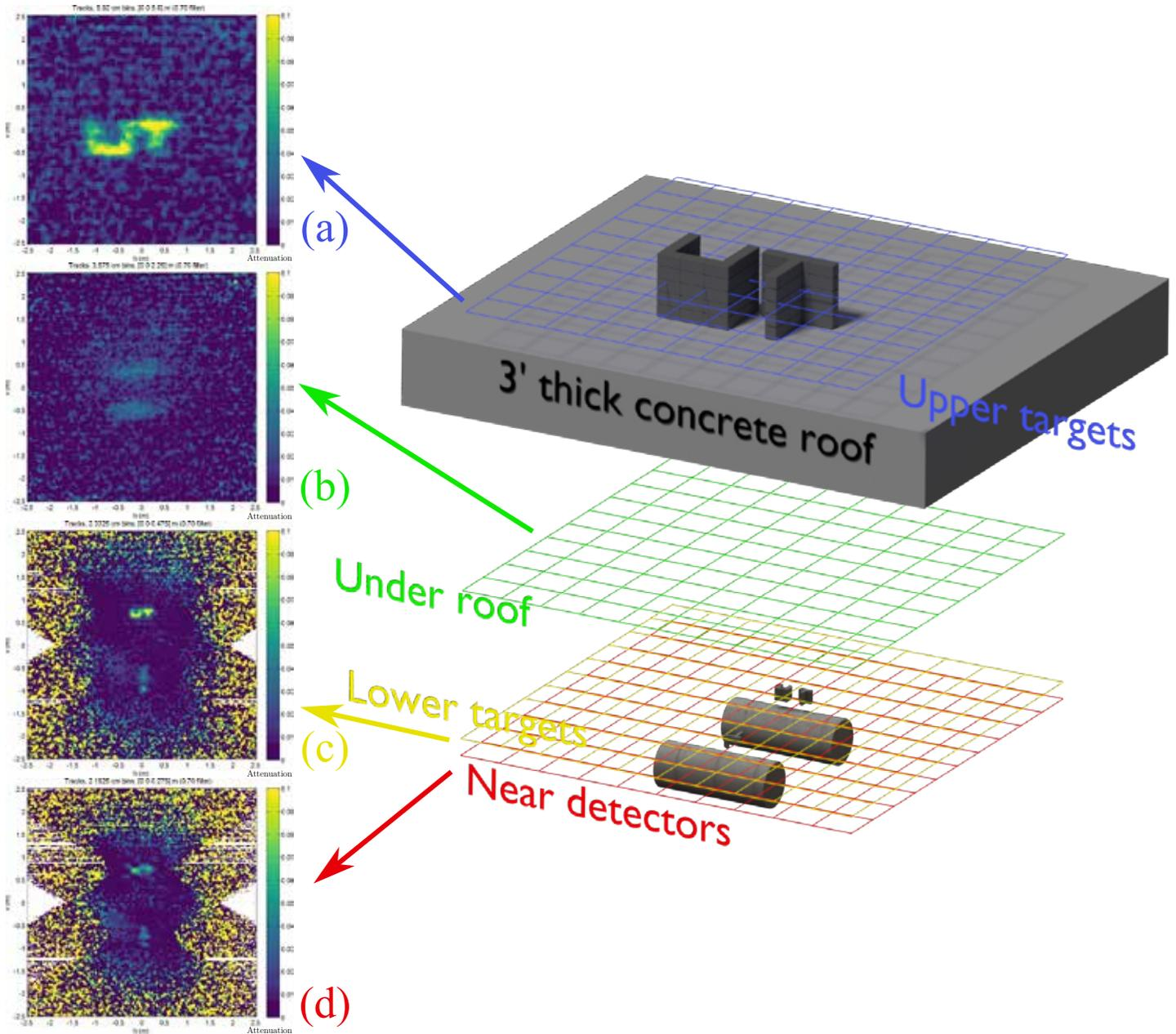
**Figure 2:** A data set collected with two horizontal detectors. Just above the detectors, 2x4x8 inch (5x10x20 cm) lead bricks were stacked in a couple of different orientations (visible in c). Above the roof of the lab a collection of lead-concrete bricks was stacked (visible in a). Projections between the targets show an out-of-focus “shadow” (visible in b ). Color scales represent attenuation of muons relative to an open sky.
