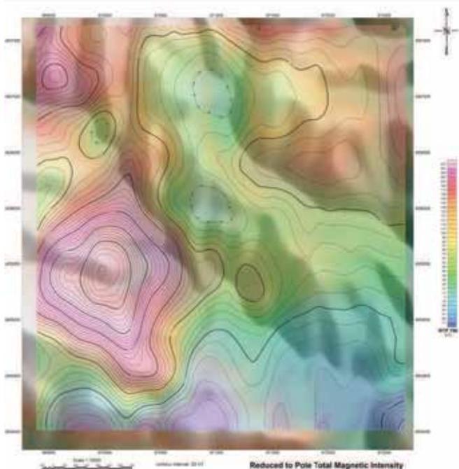
**Figure 4:** MGT UAS magnetometry data draped over DEM for mineral exploration.
