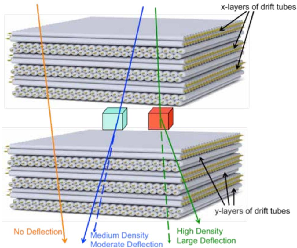
**Figure 2:** Tomographic imaging mode.
