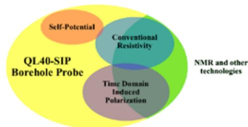
Providing a superset of measurements, the SIP probe will cost-effectively compare with nuclear magnetic resonance (NMR) logs, while also providing SP and conventional resistivity logs. It will also provide an inherently safer alternative to nuclear logging tools using radioactive material.
