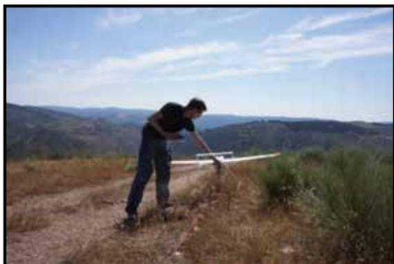
**Figure 5:** S180 Mk.2 sUAS fitted with MGT magnetometer preparing to be launched via a catapult.
