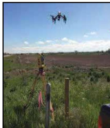
**Figure 1:** DJI Inspire 1 used by Wohnrade Civil Engineers for site characterization surveys.
