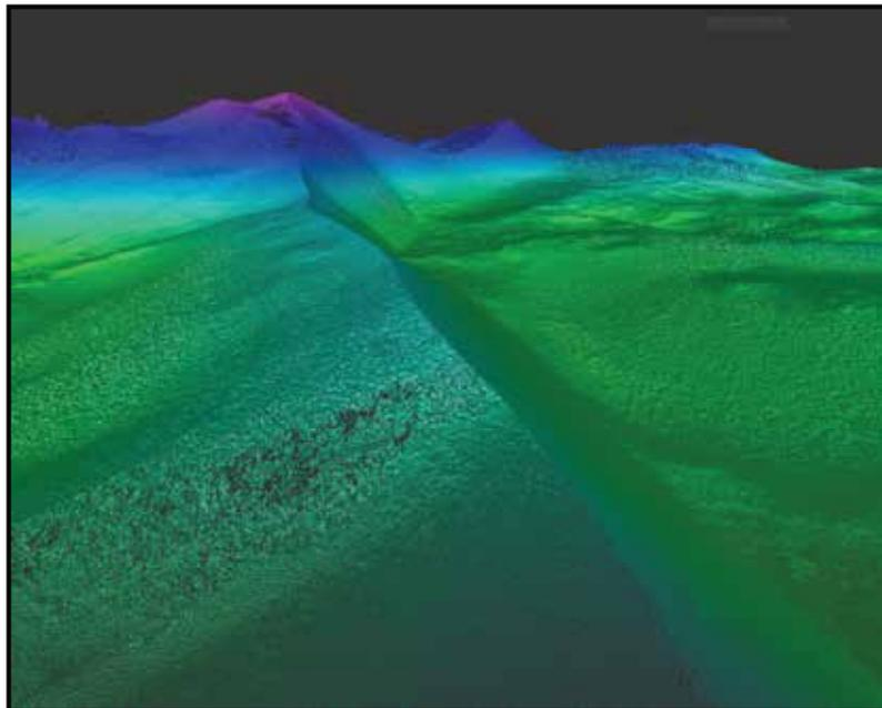
**Figure 3:** Rendering of 3D Point Cloud of digital elevation data obtained from a UAS photogrammetric survey.
