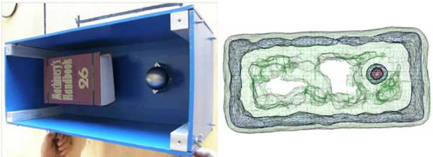
**Figure 4:** A book (low density) and a sphere of tungsten (high density) inside a lead box (left) with the corresponding muon image in 2D (right).
