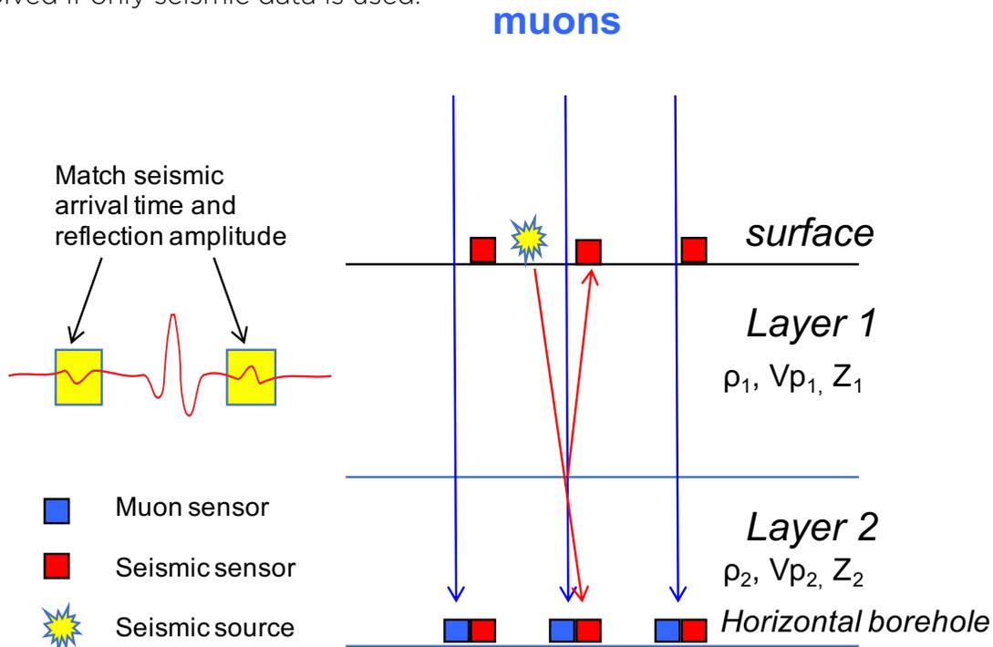
**Figure 2:** Schematic of imaging using travel-time and reflection coefficients. Here the geometry is as in Figure 1, but with additional seismic sensors on the surface, as in a seismic reflection survey. This allows measurement of the reflection from the layer interface, which provides additional constraints on the layer properties. In this case, S wave travel time are not necessarily measured.
