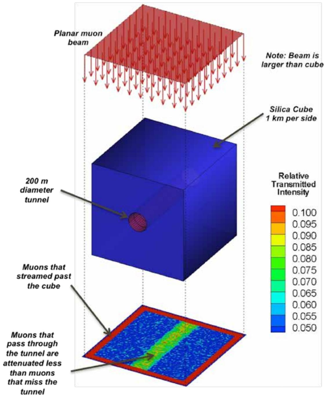
**Figure 5:** Simulation results of muon flux after passing through a cube of rock (e.g. silica) with an air-filled tunnel.
